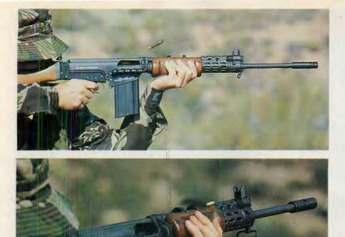
aluminum retracting handles are much larger than those encountered on other metric FALs. The takedown hinge pin connecting the upper and lower receivers has a unique configuration and requires a spanner wrench for removal. Takedown levers remain in the original position, in back of the upper receiver (they have been moved downward on current FN FALs). The magazine catch is of a peculiar ringed spur shape and the hold-open thumbpiece is the small, early FN type.
